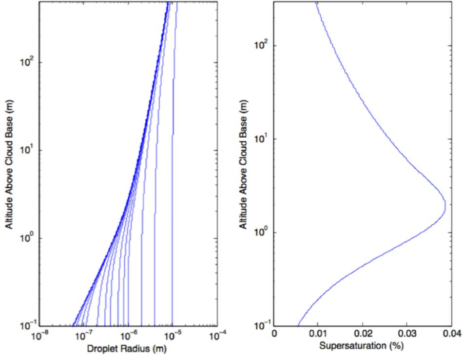
Figure 1. Evolution of a population of droplets with altitude (left). Evolution of supersaturation of an air parcel with altitude (right).
